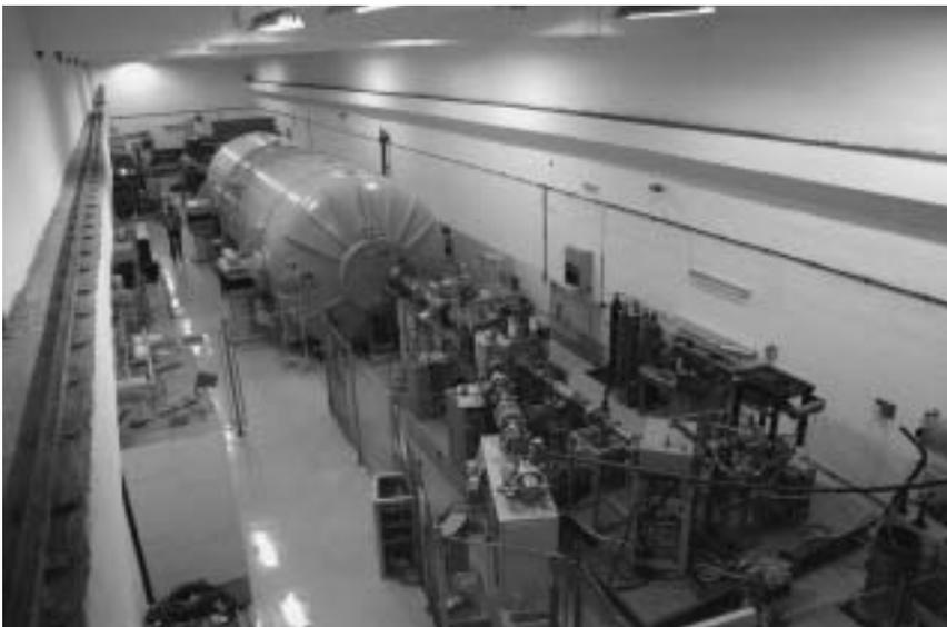
**Figure 1.** A general view of the main vault of the Bucharest 9 MV Van de Graaff Tandem Accelerator.
