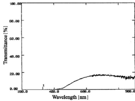
c)  $\text{Fe}_2\text{O}_3$  doped 5%Fig. 2. – UV spectra of the  $\text{Fe}_2\text{O}_3$  doped soda-lime-silica glasses.
