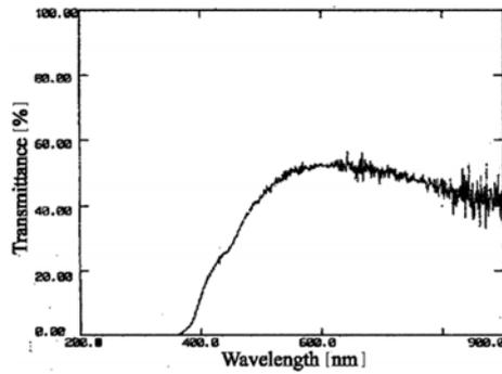
b)  $\text{Fe}_2\text{O}_3$  doped 3%
