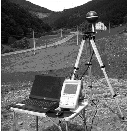
Fig. 2 – TS-EMF measurement system for frequency selective measurements.
