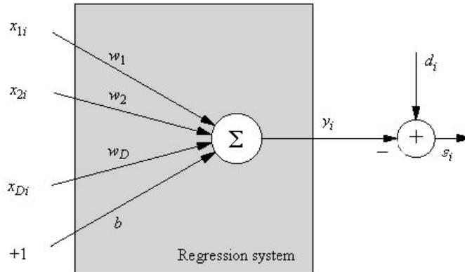
Fig. 2. – The linear Processing Element.
