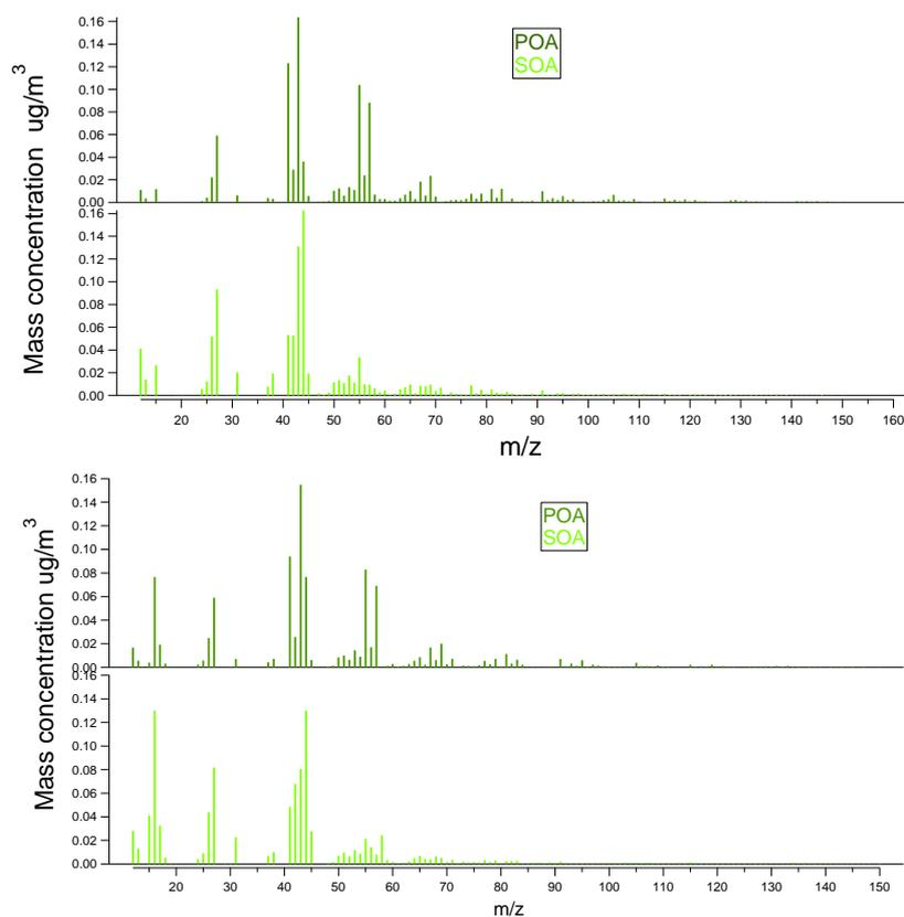
Fig. 3 – Mass spectra of organic aerosols: upper panel – fresh aerosol generated by a local fire; lower panel – aged aerosol in second day.
