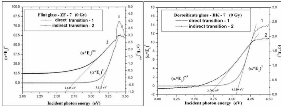
Fig. 2 – Optical band gap energy vs. incident photon energy (ZF-7 and BK-7; non-irradiated sample).
