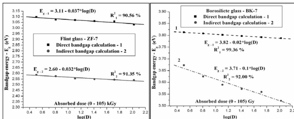
Fig. 5 – Optical band gap energy of ZF-7 (left) and BK-7 (right) glass vs. absorbed dose.
