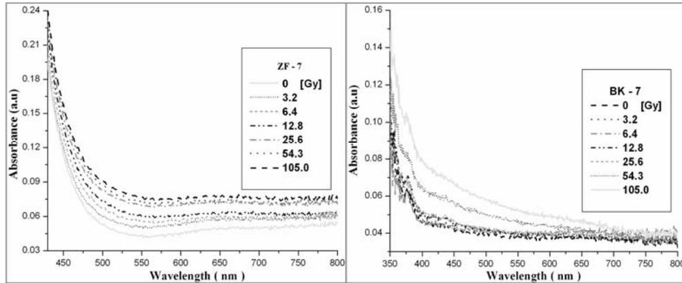
Fig. 1 – Absorbance spectra corresponding to ZF-7 (left) and BK-7 (right) studied glass types.
