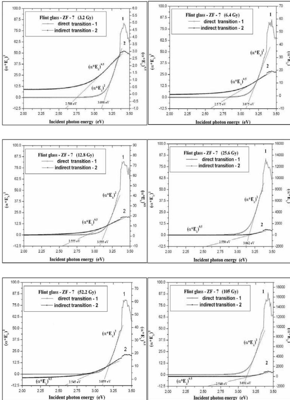
Fig. 3 – Optical band gap energy of ZF-7 glass vs. incident photon energy (the six absorbed dose values).
