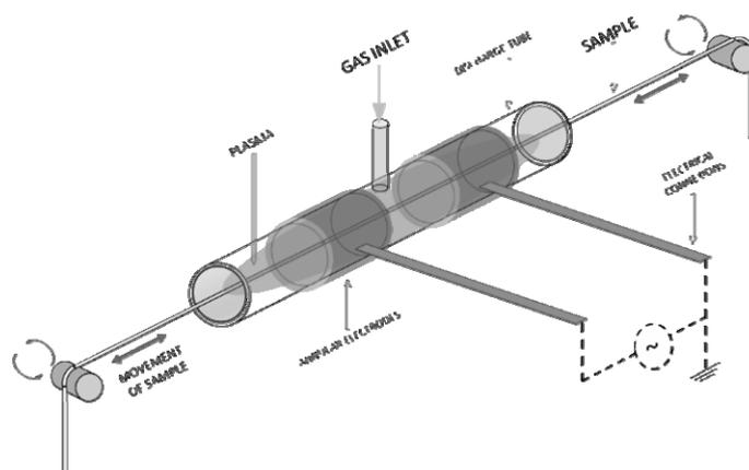
Fig. 9 – Plasma device for processing of outer surfaces of objects with small diameters.
