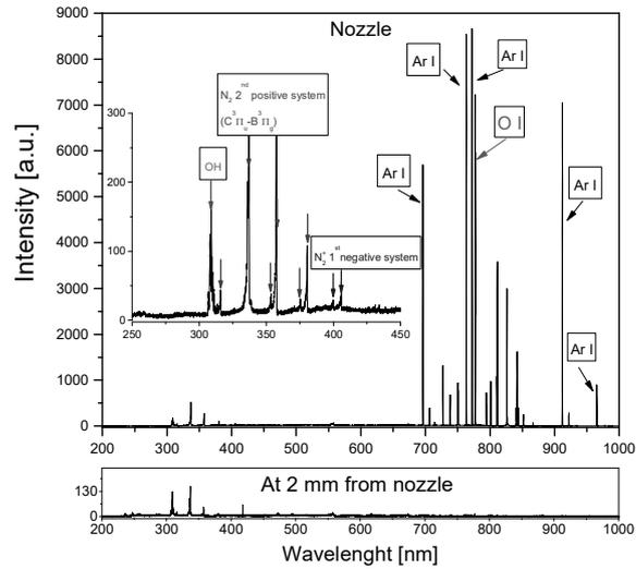
Fig. 2 – Spectra of plasma at nozzle exit (up) and 2 mm far from nozzle (down), at 14 W forwarded power and 4500 sccm argon flow rate.
