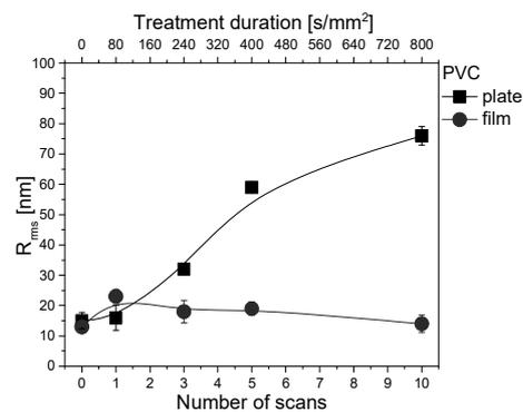
Fig. 8 – Dependence of  $R_{\text{rms}}$  for  $40 \times 40 \mu\text{m}$  upon the number of scans (bottom horizontal axis) or treatment duration (upper horizontal axis) with plasma source.
