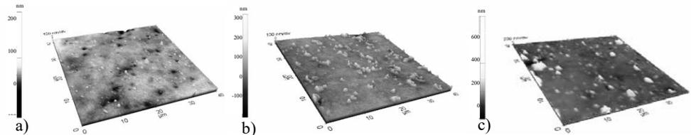
Fig. 6 –  $40 \times 40 \mu\text{m}$  AFM images (3-D) of PVC plate: a) untreated and treated with plasma; b) 5 scans and c) 10 scans.
