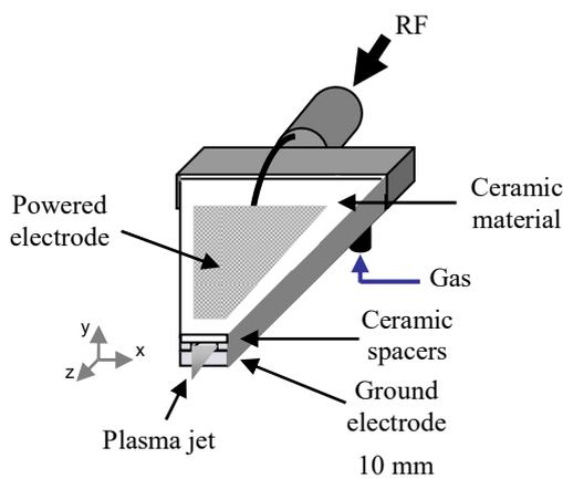
Fig. 1 – Schematic diagram of the plasma source with a single barrier and trapezoidal parallel configuration.
