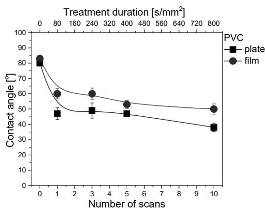
Fig. 4 – Water contact angle dependence for PVC plate and film upon the number of scans (bottom horizontal axis) or treatment duration (upper horizontal axis) with plasma source.
