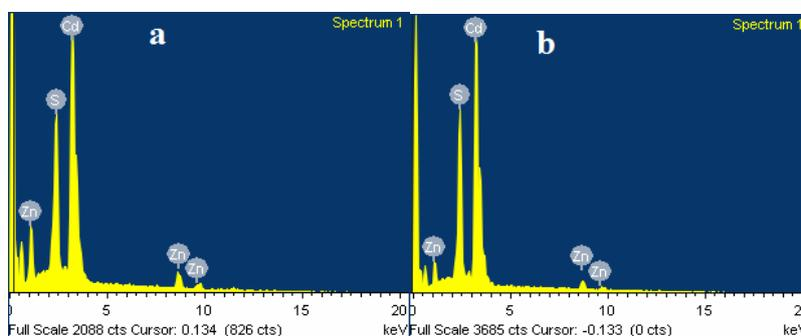
Fig. 3 – (Color online) a) EDAX image of  $\text{Cd}_{0.9-x}\text{Zn}_{0.1}\text{S}$  QDs, b)  $\text{Cd}_{0.9-x}\text{Zn}_{0.1}\text{Li}_{0.02}\text{S}$  QDs
