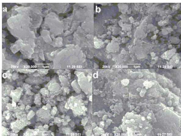
Fig. 2 – (Color online) SEM images of  $\text{Cd}_{0.9-x}\text{Zn}_{0.1}\text{Li}_x\text{S}$  samples.
