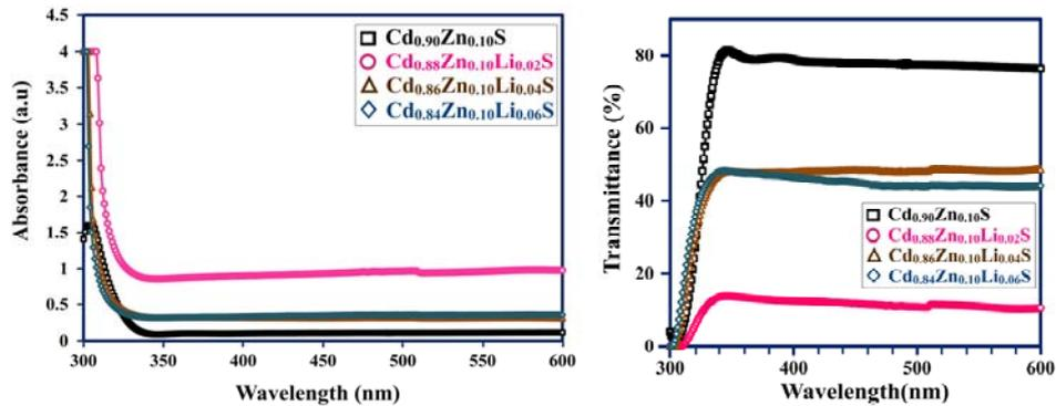
Fig. 4 – (Color online) UV-Vis spectra of  $\text{Cd}_{0.9-x}\text{Zn}_{0.1}\text{Li}_x\text{S}$  samples: a) Absorbance, b) Transmittance.
