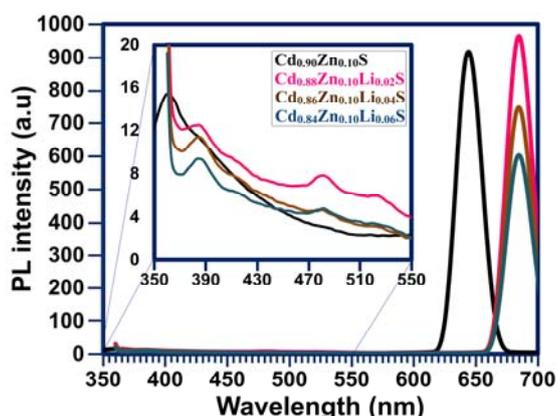
Fig. 5 – (Color online) Photoluminescence spectra of  $\text{Cd}_{0.9-x}\text{Zn}_{0.1}\text{Li}_x\text{S}$  samples.
