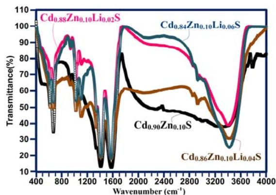
Fig. 6 – (Color online) FT-IR spectra of  $\text{Cd}_{0.9-x}\text{Zn}_{0.1}\text{Li}_x\text{S}$  samples.
