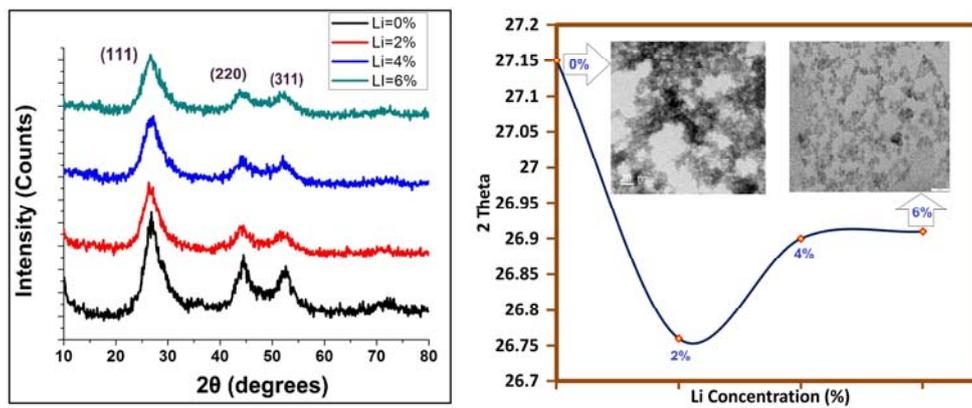
Fig. 1 – (Color online) a) XRD patterns of  $Cd_{0.9-x}Zn_{0.1}Li_xS$  samples, b) Variation of particle size vs Li concentration.
