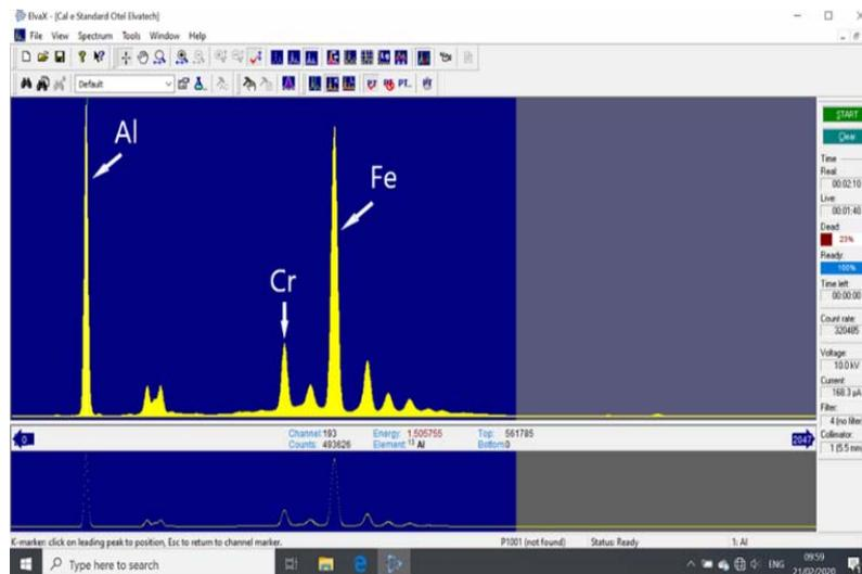
Fig. 2 – XRF spectra for a 316 Steel calibration standard.
