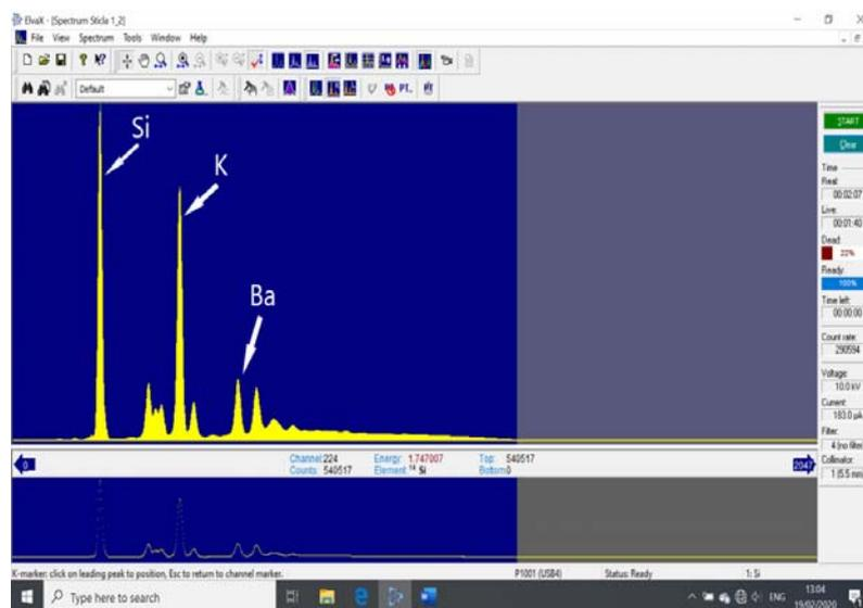
Fig. 3 – XRF spectra for a BK7 glass sample.
