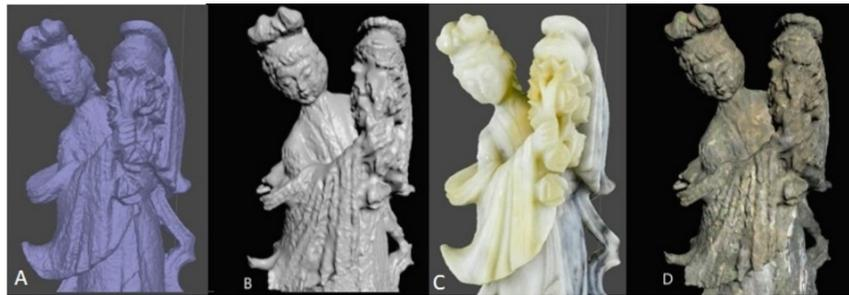
Fig. 4 – (Color Online) Visual comparison of the jade statuette generated 3D models: A, C – photogrammetry, B, D – laser scan.
