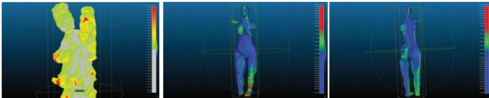
Fig. 6 – (Color Online) Calculated differences between the laser scan and photogrammetry 3D models for each object.
