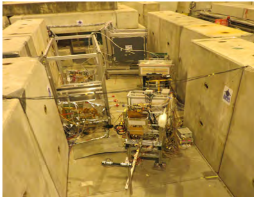
Fig.36 A photo of the experimental configuration for the in-beam tests at SPS of the new generation of high counting rate MSMGRPC (Multi-Strip Multi-Gap Resistive Plate Counters) and TRD-2D (Transition Radiation Detectors) with 2 dimension position information and associated frontend electronics developed by members of Hadron Physics Department for the CBM experiment at FAIR (Facility for Antiprotons and Ion Research), Darmstadt, Germany.
