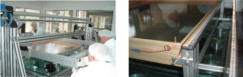
Alignment of multiwire electrodes.
