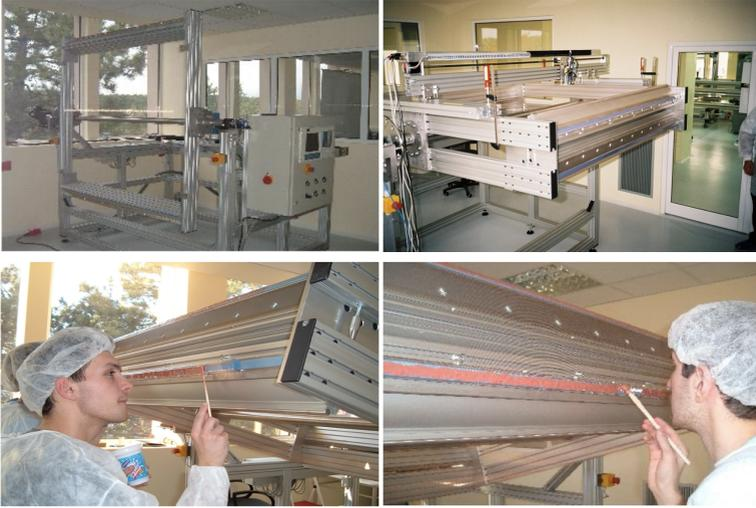
Winding and gluing of multiwire electrodes.
