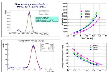
Energy resolution and gain tests.
