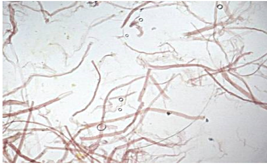
Fig.1 Photomicrograph (x200) of rag fibers treated with Graff 'C' stain found in original paper of old printed books Menology for May and The Bible .
