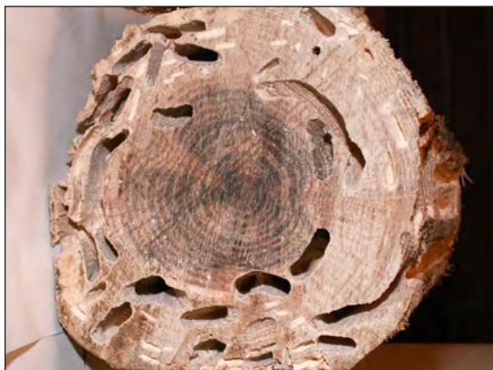
Fig. 2: Larvae tracks in wood
