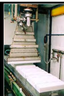
Irradiated objects are placed on the conveyor, which transfers the sweeping them under the electron beam. Time treatment is very short - a few seconds. Elektronika 10/10 electron accelerator (Institute of Nuclear Chemistry and Technology, Warsaw Poland)
