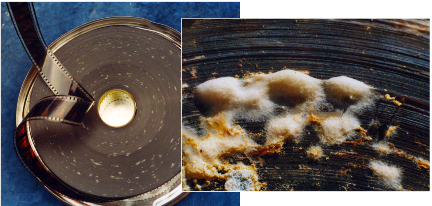
Fig. 28: Contaminated pellicule, Romanian Film Archive
