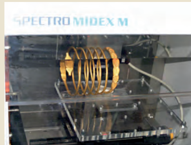
XRF Fixed Spectrometer: SPECTRO MIDEX M (Rhodium anode); Dacian gold spiraled bracelet - 13 bracelets: Au=8 4.2-92.9% ; Ag=6.3-16.2%; Cu=0.4-2.1% Alluvial gold (Valea Pianului - Alba County) mixed with surface vein gold (Valea Morii - Apuseni Mountains)
