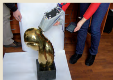
XRF Portable Spectrometer; alloy of a Mlle Pogany III statuette type presumably belonging to Brâncuși: brass (Cu=75%, Zn=19%, Sn=3%, Pb=1.7%); used by Susse Fonderie, Paris, around 1960. The brass used at Valsuani Fonderie, Paris, by Brâncuși during his life is different from this one (Cu=82%, Zn=12.5%, Sn=4%, Pb=0.4%)
