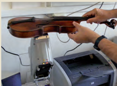
XRF Portable Spectrometer; pigments and varnish of a presumed Stradivarius violin: a lead-based pigment (XVIIth - XVIIIth centuries) and in some areas a chromium-based pigment (XXth century) from a repainting
