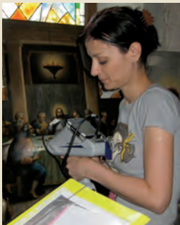
XRF Portable Spectrometer; pigments of mural painting and iconostasis of Măgurele Church - Ilfov County; painted by Gh. Tătărescu, 1853: red-cinnabar, lead white with white zinc from a XXth century repainting, ochre, iron blue, chrome-yellow, gold-powder mixed with "bolos" - a special type of ochre
