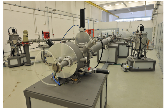
Fig. 2. The 3 MV Tandetrion accelerator at IFIN-HH. NA measurements were done on the beam lines in center and at right.
