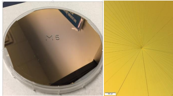
Figure 1. Helical mirror and the central part for the topological order l=5
