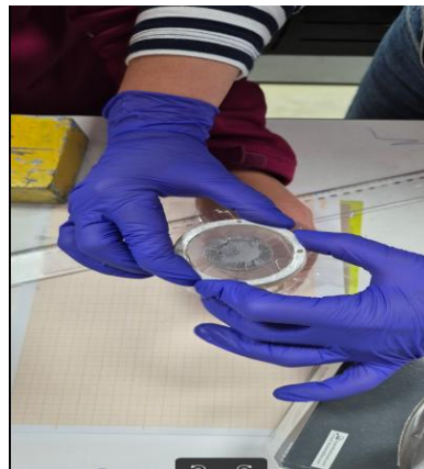
Figure 3: Preparation of the ^{28}\text{Si} sample in the target laboratory of IFIN-HH.
