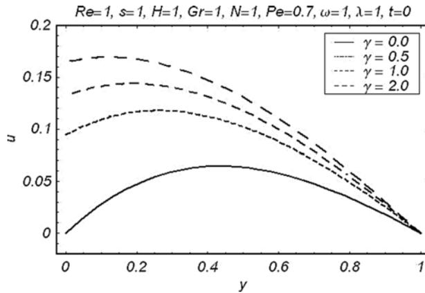
Fig. 1 – Effect of wall slip on the velocity  $u$ .
