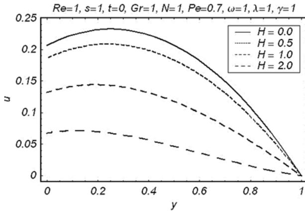
Fig. 4 – Velocity curves for different values of the Hartmann number  $H$ .
